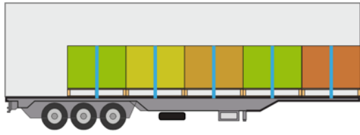
Locked blocked in forward direction and tied down for lateral and rearward restraint
