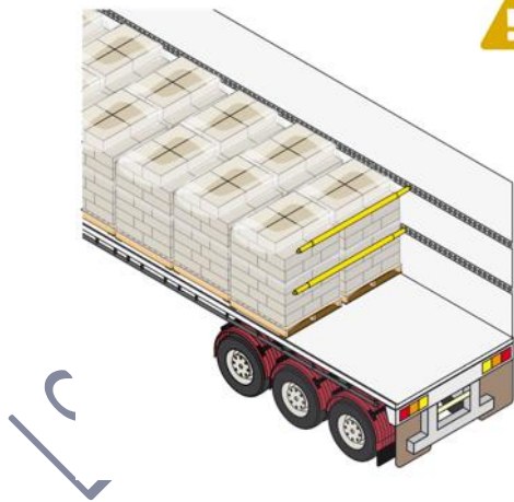
Only use shoring/blocking bars to stabilise loads because they have limited load restraint capacity. Rated bars may be suitable for blocking some loads.
